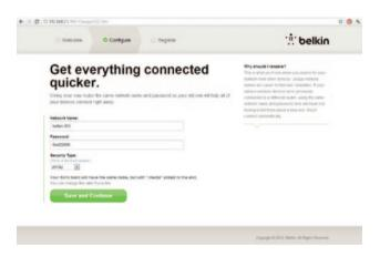
At the next screen you will be invited to change your network name and password. Reusing your previous network name (SSID) and password makes connecting your existing devices to the new Modem Router much easier.
